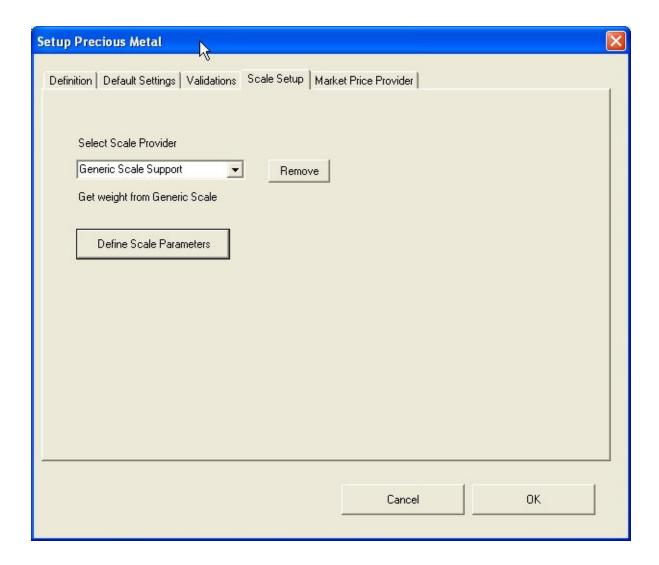
Scale Parameters – Port settings and Command script can be retrieved from the scale documentation. The command should return the Weight followed by the Weight Units followed by a termination character. Use the TEST button to test the command.
